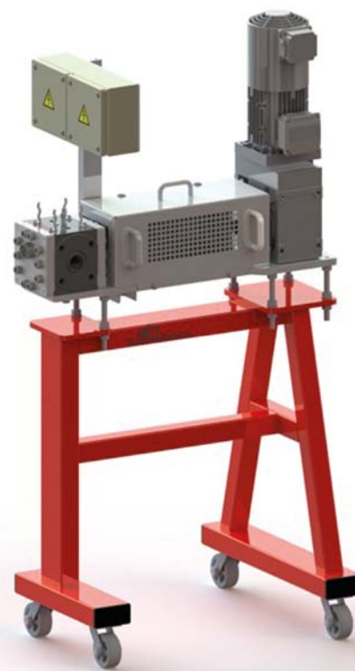
Melt Pump Unit with Drive and Support Cart
